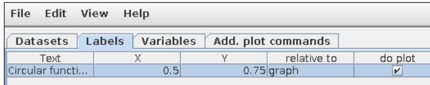
The previous screenshot shows the window that we used for adding the label **Circular functions**. These windows are accessed by clicking on the tabs that can be seen in the large main window.
