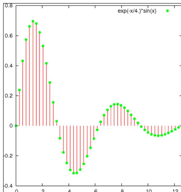
As you can see, we have plotted the same function twice. The first time through plot the impulses, as in the previous script, and the second time we plot the function again with points to draw the dots.
