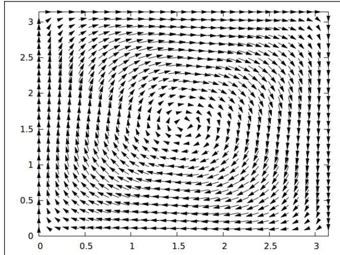
The previous figure is a vector field of a rotating flow. The exact appearance of the arrows will vary with the output terminal.
