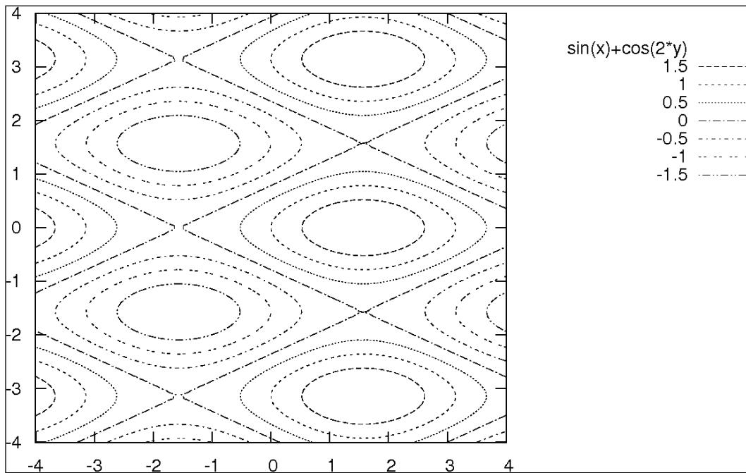
Certain types of patterns are better represented as surfaces, while for others, contours bring out more of the relevant characteristics. The rotationally invariant function that we plotted in the previous recipes in this chapter would yield a set of uninteresting circular contours; its structure is better conveyed by a surface plot. Here, we've plotted a function whose contour plot shows a pattern of nodal lines.
