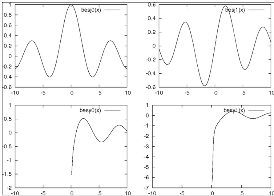
In the previous figure, we have made a table of graphs showing the four kinds of Bessel function that gnuplot has built in.
