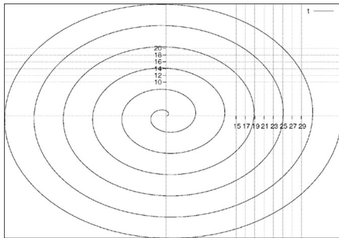
The previous figure is similar to the one towards the end of *Chapter 1, Plotting Curves, Boxes, Points, and more*, where we introduced polar coordinates. The difference here is that we have placed our tic marks only in a certain area—that you can imagine is a region of interest—and added grid lines so the reader can more easily extract quantitative information from the graph in the region.
