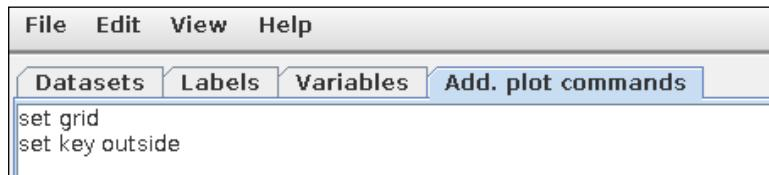
We used this to set the parameters for the key and the grid; this window is for adding commands to the plot script that are not directly accessible from the GUI.
