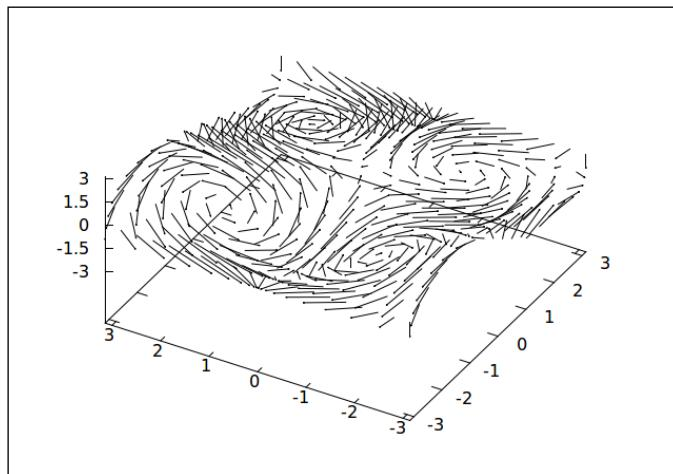
The vectors are plotted on an imaginary surface that is not depicted explicitly. Experimentation shows that the arrowstyle cannot be changed by the user, despite the documentation, but depends only on the terminal. This type of plot can be used, for instance, to describe a fluid flow in 3D; the contrived example shown was chosen to make the script easy to understand:
