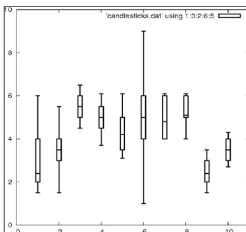
In the previous plot, typically, the boxes show the range of the central part of the data distribution; the short horizontal line within the boxes shows the value of the mean; and the vertical lines extending above and below the boxes show the range of the bulk of the distribution excluding the outliers.
