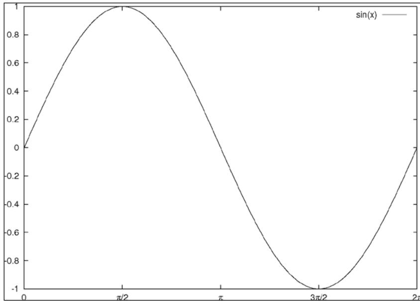
Note the appearance of Greek letters in the tic labels, where before we spelled out *pi*. We constructed these labels using the enhanced text syntax that was introduced in *Chapter 2, Annotating with Labels and Legends* as shown in the following script:
