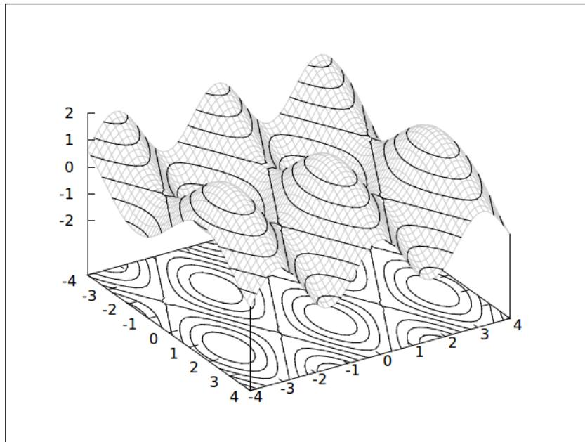
This is a plot of the same function as shown previously, with a contour plot on the base, a surface, and another set of contours drawn on the surface. Here is the script:
