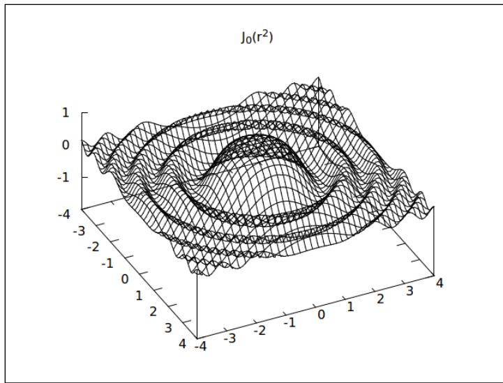
The previous figure is a perspective drawing of a surface representing the Bessel function  $J_0(r)$ , where  $r$  is the distance from  $(x=0, y=0)$ . The height of the surface shows the value of  $J_0$ , given on the vertical axis (unlabeled in this figure, but usually called  $z$ ). The other two (unlabeled) axes defining the plane above which the surface is drawn are the  $x$  and  $y$  axes.
