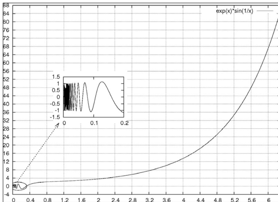
In the previous figure, the smaller plot is usually called an **inset**. We can create this figure with the script given in the following *How to do it...* section.
