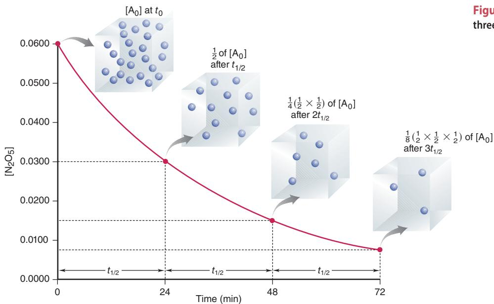
**Figure 16.12** A plot of  $[N_2O_5]$  vs. time for three reaction half-lives.
